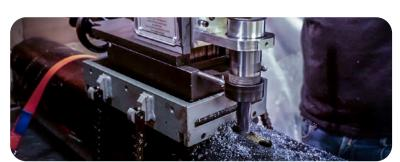
Drill and mill pipes with optional pipe cradle attachment (Part number JEICB-M).
